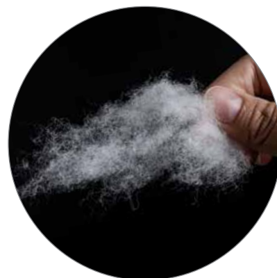
Cotton sample gently pulled apart for visual inspection of fiber length and impurities
